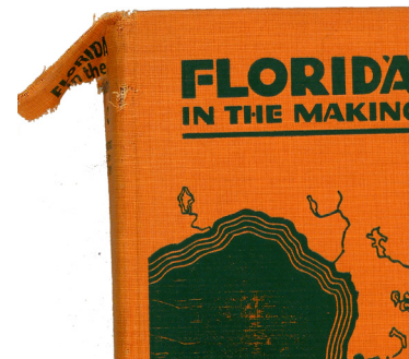
Spine piece torn by pulling on the head-cap.
